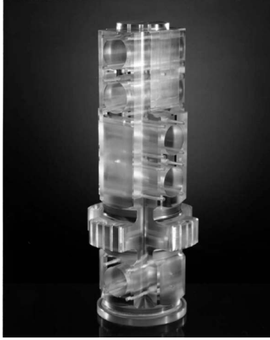
Fig. 8.5. Gravity Probe B carries four gyroscopes, mounted in a single quartz bloc, a prototype of which is shown here. The pointing telescope (not shown) is attached to the flange at the lower end. The whole unit is placed in a much larger helium dewar. Image credit: Gravity Probe B, Stanford University.
