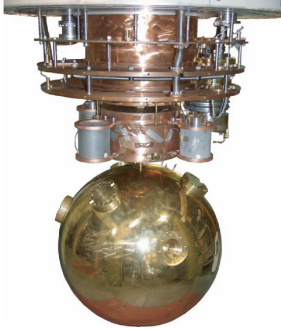
Fig. 7.7. Close up of the MiniGRAIL detector under development in Leiden. It consists of a CuAl sphere of 68 cm diameter suspended by a thin rod. The resonance frequency is 2.9 kHz, the bandwidth 230 Hz. The sphere carries several transducers that mechanically amplify and detect the vibration. The theoretical sensitivity of this 20 mK cryogenic detector is \sim 4 \times 10^{-21} . A spherical detector can determine the direction \mathbf{n} of the incoming wave (up to a \pm \mathbf{n} uncertainty) because the relative excitation levels of the quadrupole modes of the sphere depends on \mathbf{n} . Image credit: A. de Waard and G. Frossati. See http://www.minigrail.nl/
