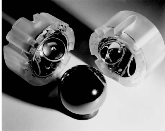
Fig. 8.4. Inside view of a gyroscope of Gravity Probe B and its housing. The rotor has a diameter of 3.8 cm, and is made of fused quartz coated with niobium. Image credit: Don Harley.
